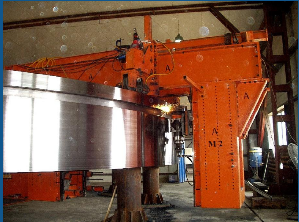
On-Site Machining by Self Leveling Machines (SLM)
