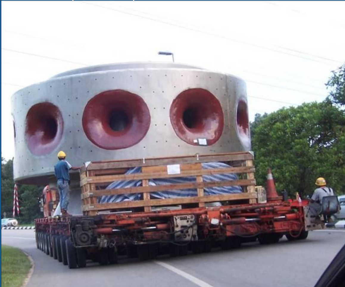
ATP Processor Centre Support – Offloading From Ship and Road Transport Inside China (Fabricated in Malaysia)
