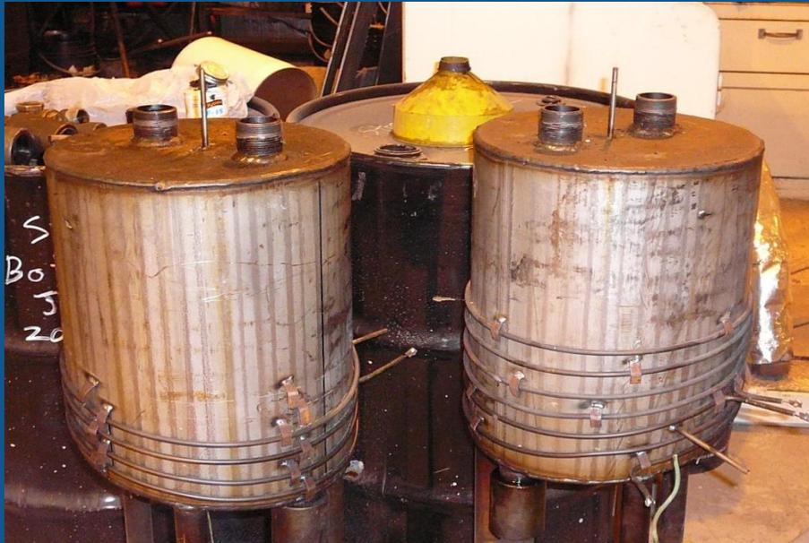
Pictured on the left are stainless steel containers used for the slow soak tests
