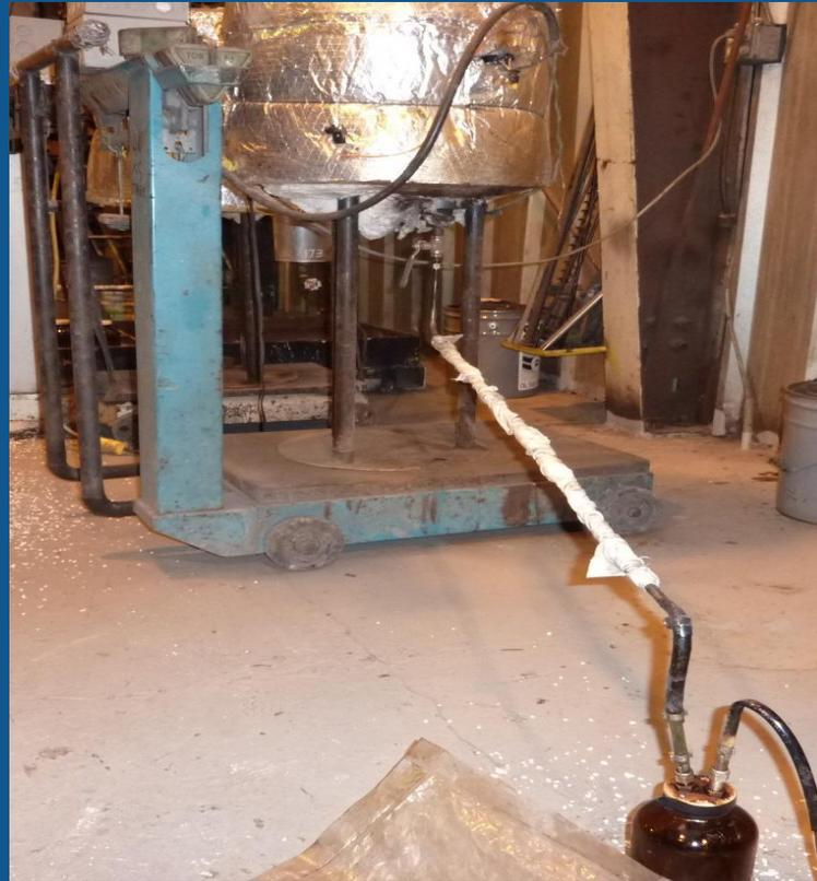
Test Series D tests were carried but with vapour bottom discharge to eliminate effects of oil condensing and refluxing back into hot oil shale charge. Only Jordan and Utah oil shales tested to date.
