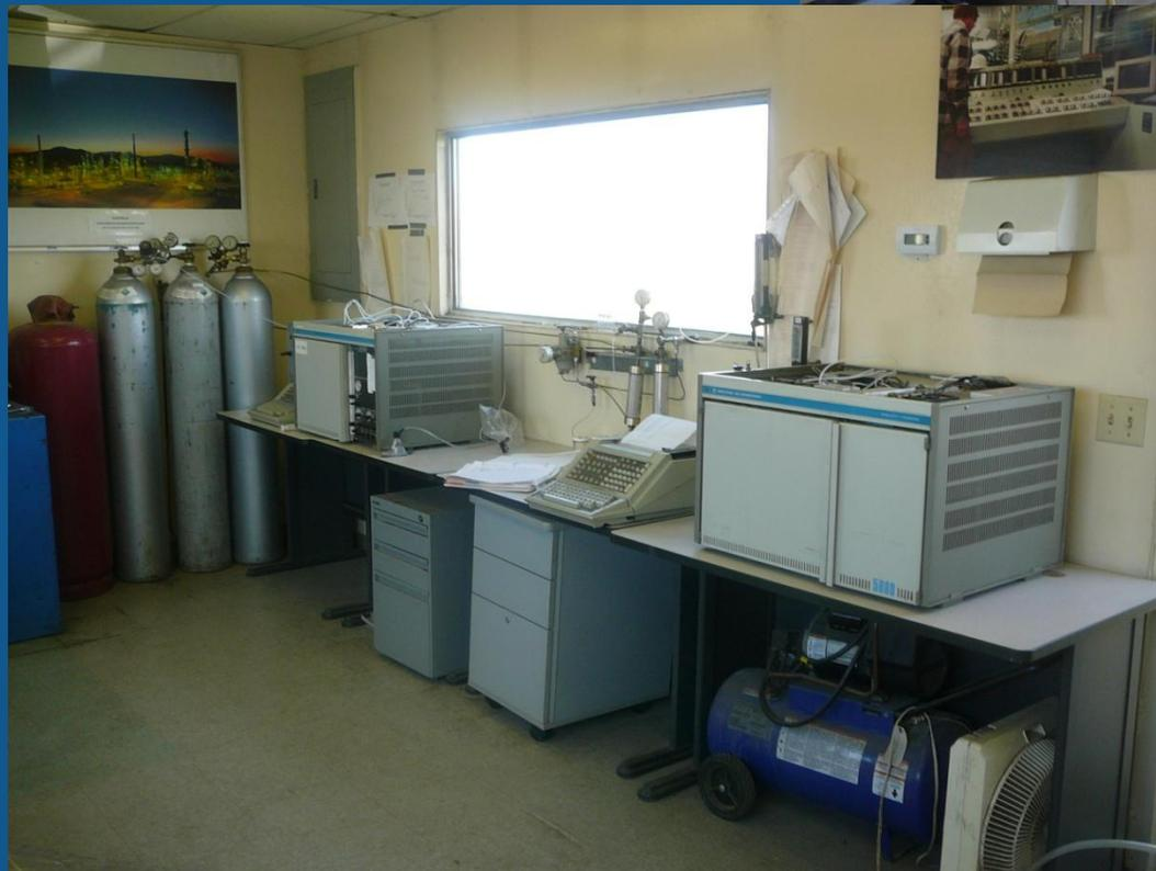
Shown on the left are UMATAC's gas chromatographs – one is used to measure refinery gas and the other for hydrogen and methane
