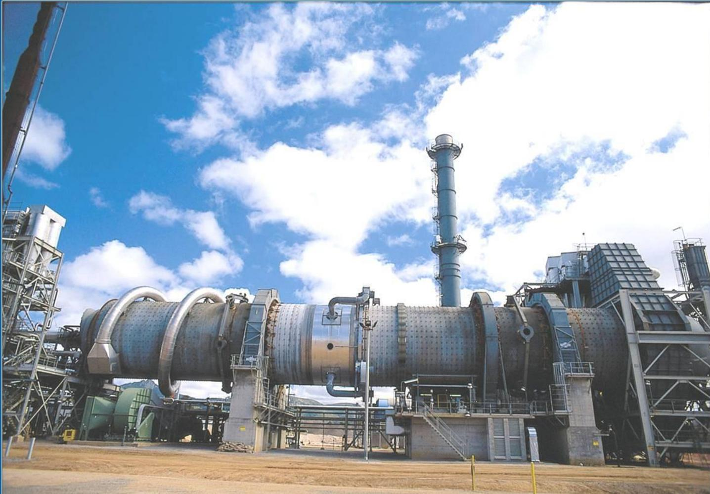
211 t/h ATP Processor at the Stuart Oil Shale Demonstration Facility
