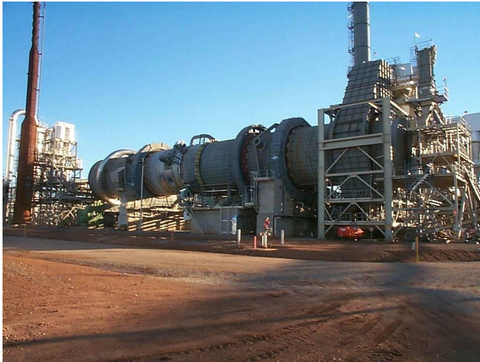
Stuart Project Alberta Taciuk Processor, 8.2m diameter x 63 m long
